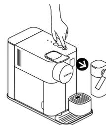
**4** Press the milk button for 3 seconds to enter Menu mode: descaling and clean alerts start blinking.
